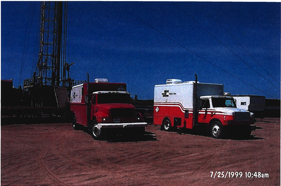
Photograph 9 – Lake Meredith Salinity Control Project: Baker Hughes logging trucks are set up to do cement bond logging of surface casing at Injection Well No. 1. Photographed 7/25/1999 by Dennis McDonough.
