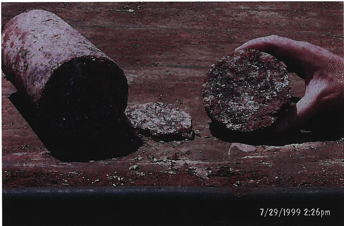
Photograph 14- Lake Meredith Salinity Control Project – White crystals of halite (salt) appear in core removed from the bit and reaming shell. This core is from the bottom of the cored interval 2155 to 2185 ft in Injection Well No. 1. Photographed 7/29/1999 by Dennis McDonough.
